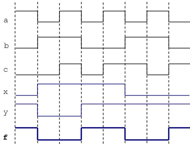
c) The following is the timing diagram of a logic circuit with 3 inputs. Sketch the logic circuit that generates this waveform. Then, complete the VHDL code. (8 pts)
